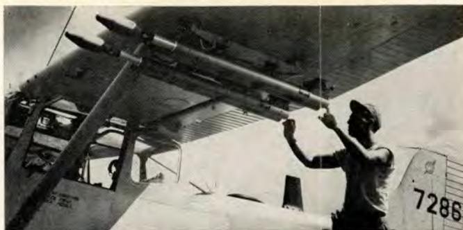
White phosphorus grenades fired from O-1's spot targets for fighter bombers. Sighting system is primitive.
